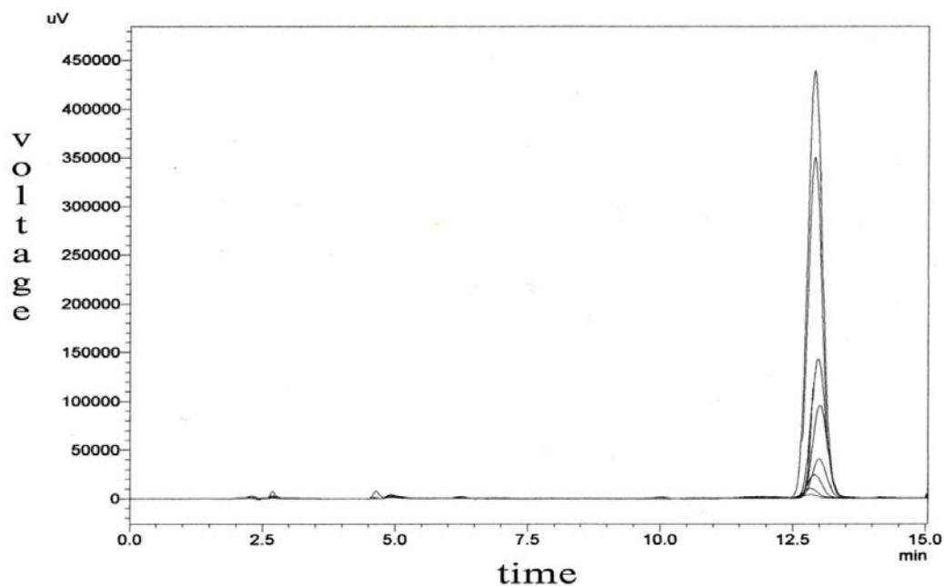
Figure 2. Chromatograms of standards solutions with different concentrations of chlordiazepoxide
