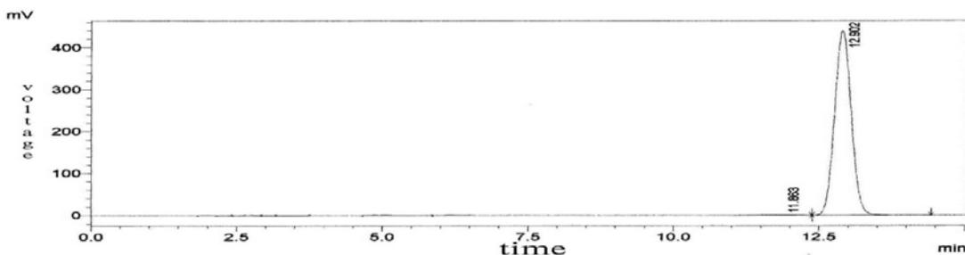
Figure 4. Chromatogram of standard chlordiazepoxide
