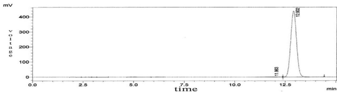
Figure 1. Chromatograms of validation of the method for chlordiazepoxide
