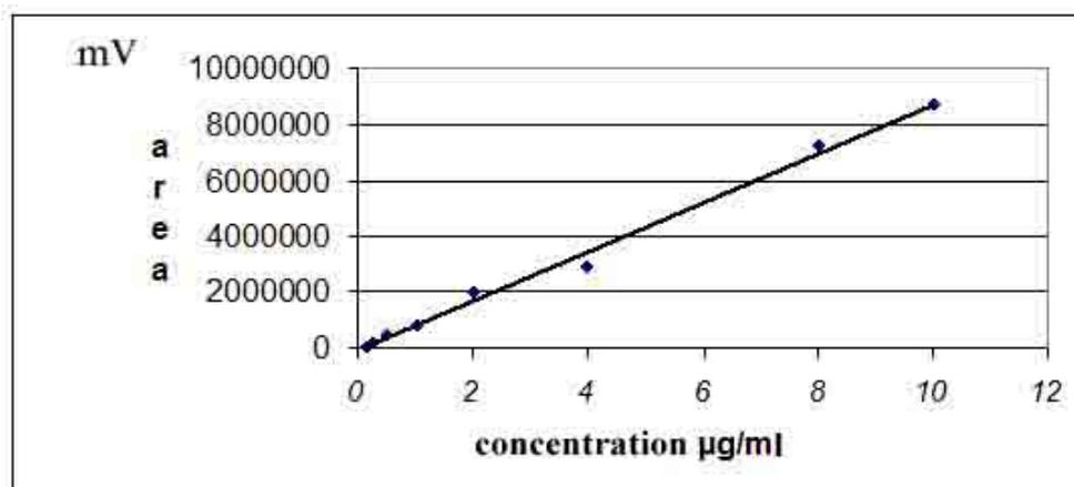
Figure 6. Calibration plot for chlordiazepoxide standards on X axis concentration ( $\mu\text{g/ml}$ ) and on Y axis peak area (mV)
