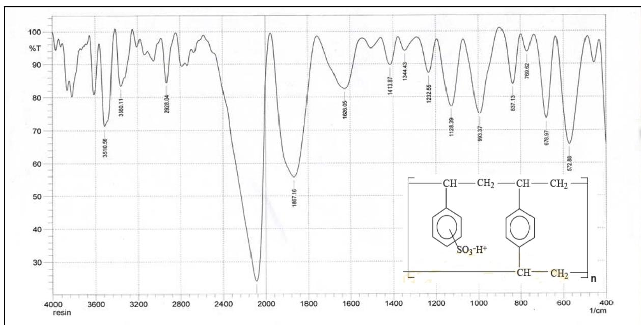
Figure 2: IR spectrum of dowex® 50 wx4
