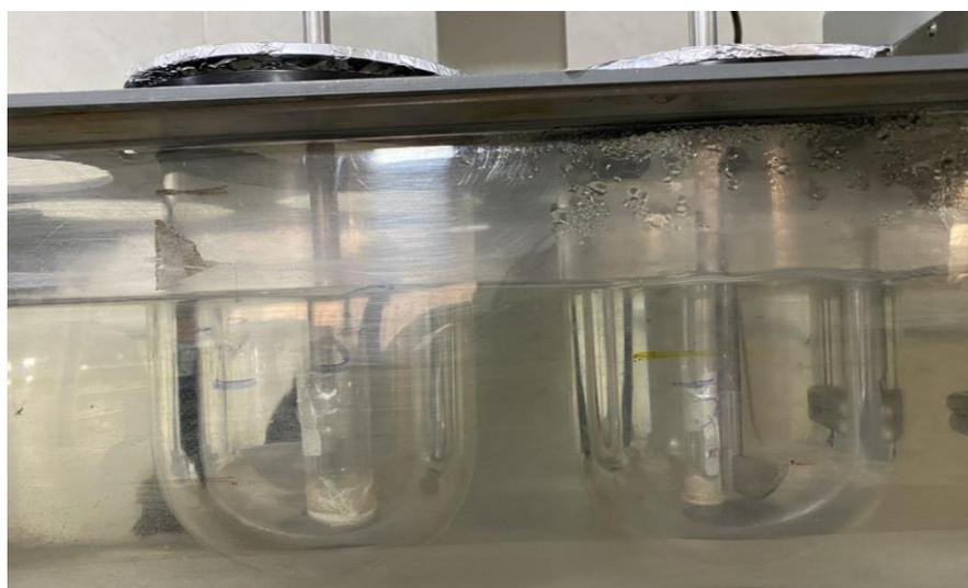
**Figure 2:** The modified method (dissolution apparatus II) of *ex vivo* skin permeation study.
